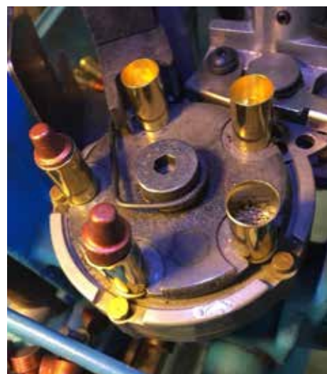
LOADING .45 CS USING .45 ACP DIES AND .45 COLT SHELL PLATE, APP FFFG.
