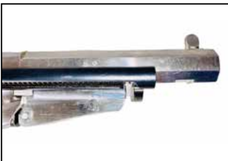
KIRST EJECTOR MODIFIED TO USE A COLT EJECTOR ROD.
