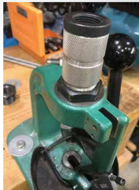
ROCK CHUCKER PRESS WITH 7/8" BUSHING AND WITH BUSHING REMOVED AND SIZING DIE IN PLACE.
