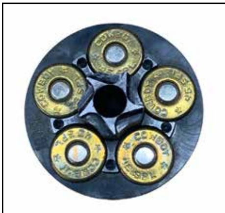
LOADED CYLINDER. NOTE HAMMER FIRING PIN RETAINERS BETWEEN CHAMBERS.
