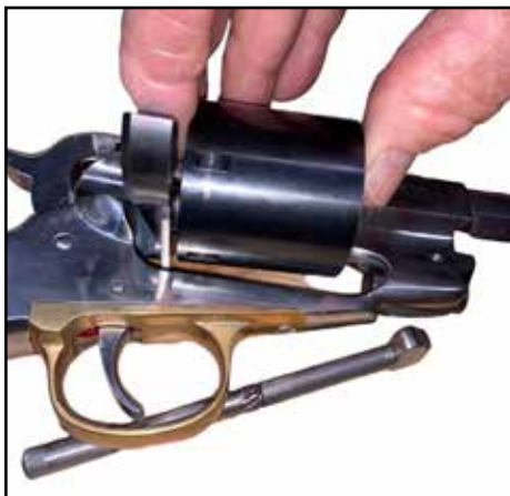
THE CYLINDER DROPS IN EASILY IF ALIGNED. THE FLAT, VISIBLE, MUST BE ON THE BOTTOM.
