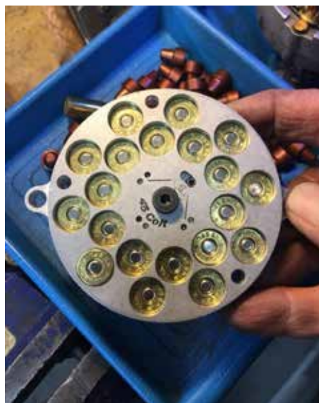
ST MACHINING .45 COLT CHAMBER CHECKER (COWBOYBULLETS.COM). ALL THE CARTRIDGES HAVE PASSED.
