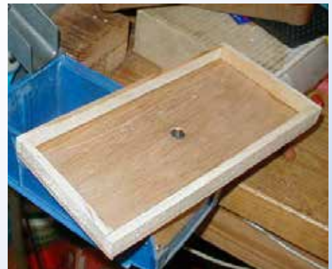
A VIEW OF HOW THE SCREW FITS FLUSH WITH THE BOTTOM OF THE TRAY.
