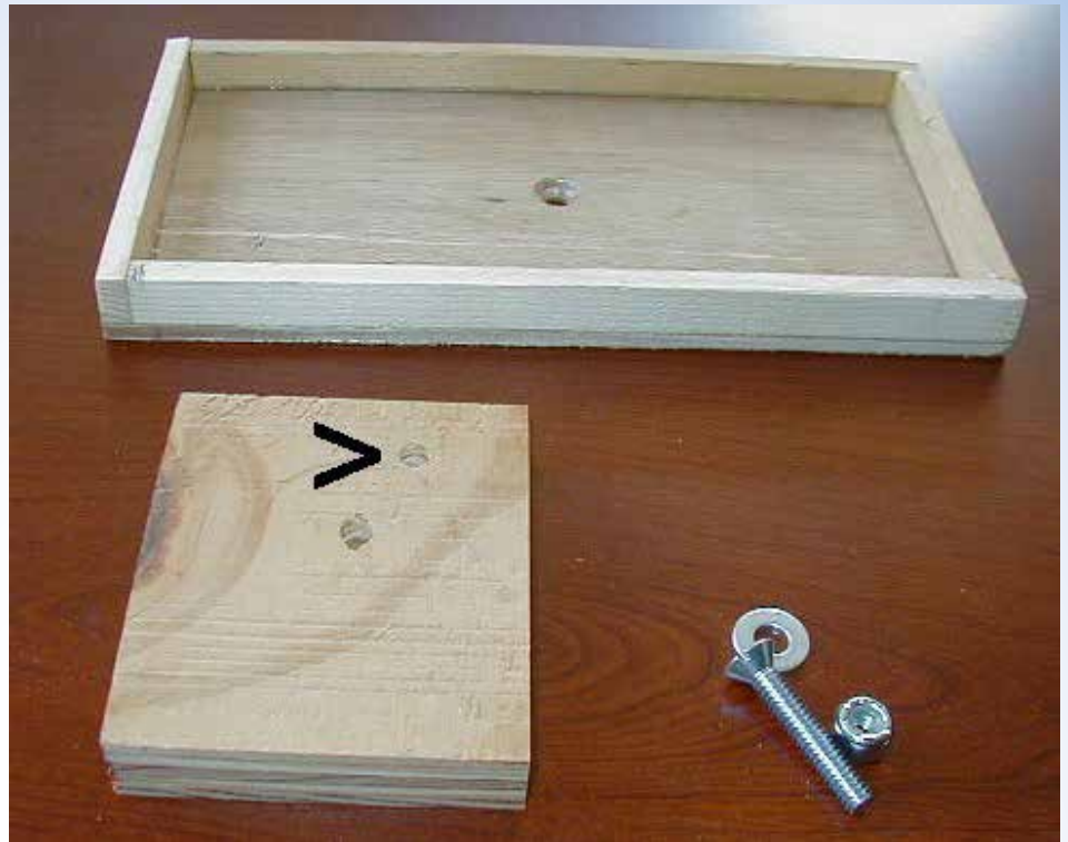
THE MAIN COMPONENTS — THE WOODEN TRAY, THE BLOCK THAT FITS INTO THE BIN AND KEEPS THE TRAY IN PLACE, AND THE SCREW AND BOLT THAT ALLOWS ROTATIONAL MOVEMENT OF THE TRAY. THE TRAY IS COUNTERSUNK TO KEEP IT FLAT SO THE LOADING BLOCK WILL SIT FLAT. THE BLACK ARROW SHOWS THE HOLE'S FINAL LOCATION.
