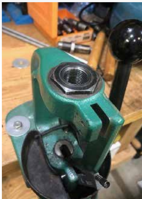
ROCK CHUCKER PRESS WITH 7/8" BUSHING AND WITH BUSHING REMOVED AND SIZING DIE IN PLACE.
