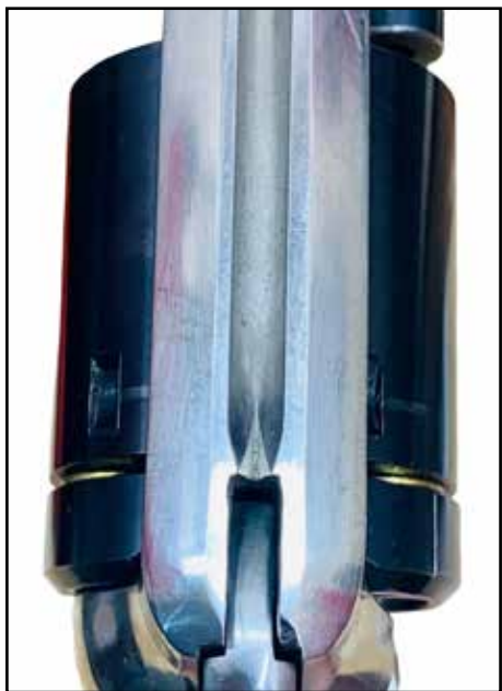
HAMMER DOWN BETWEEN CHAMBERS. BOLT LOCKS CYLINDER.
