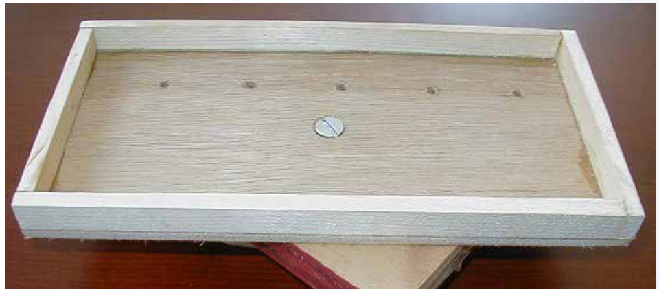
THE COMPLETED ASSEMBLY. THE RED EDGE OF THE LOWER BLOCK HELPS IN PLACING THE BLOCK IN THE CORRECT ORIENTATION ON THE BIN, REMEMBER ITS HOLE IS NOT CENTERED. IGNORE THE ROW OF HOLES IN THE TRAY—I USED SCRAP WOOD. THOSE EAGLE-EYES AMONG YOU HAVE ALSO NOTICED THE CORNERS ARE NOT ALL THE SAME. THIS WAS DUE TO THE WAY THE WOODEN STRIPS WERE ATTACHED, AS THE LOADING BLOCK ITSELF WAS USED TO DETERMINE THE SIZE OF THE TRAY.
