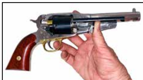
TAYLOR'S '58 REMINGTON WITH KIRST GATED CONVERSION CYLINDER WITH MODIFIED EJECTOR BY GOON'S GUNWORKS.
