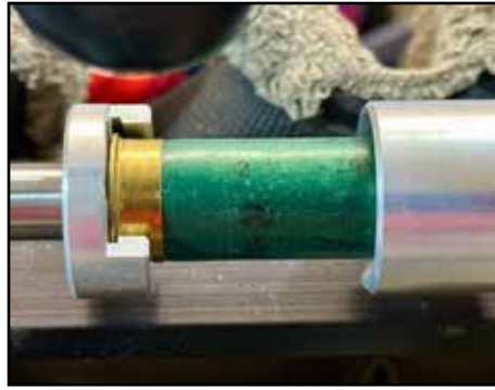
BOLT CLOSED, ROUND RESIZED AND TAPERED.
