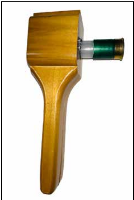
UNLOAD-IT TOOL (BALLISTIC PRODUCTS) FOR DISMANTLING SHELLS FOR RECYCLING. POWDER, WADS, AND SHOT CAN BE RECYCLED, AND PRIMERS IF YOU DARE TO DE-PRIME A LIVE ROUND.
