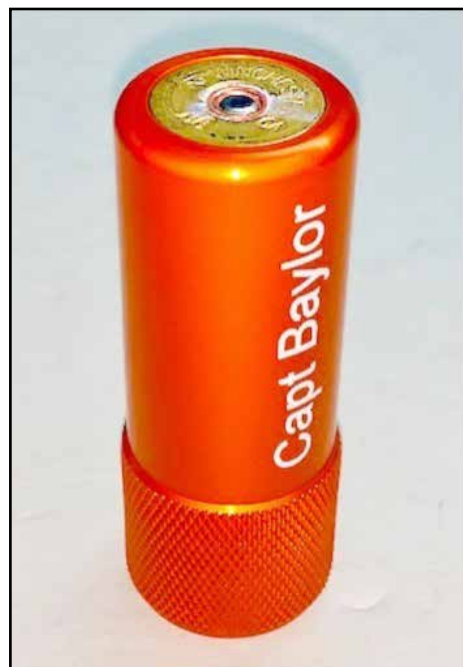
SLIX CHECKER/SIZER HAS THE SAAMI DIMENSIONS OF A 12 GAUGE CHAMBER ON ONE END AND A 12 GAUGE SIZER ON THE OTHER END FOR FIXING OUT OF SPEC ROUNDS.
