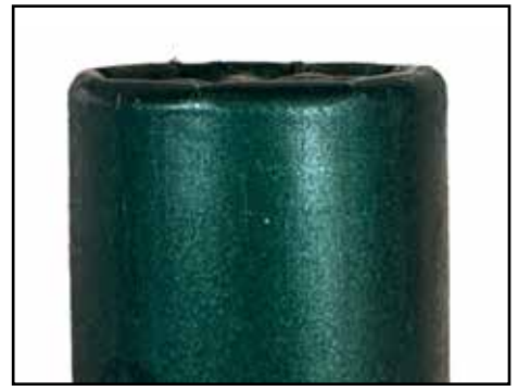
SIZED AND SLIGHTLY TAPERED ROUND. EDGE OF CASE MOUTH IS ROUNDED.
