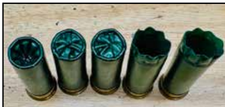
FIVE BAD ROUNDS. L-R, RECYCLE, “PRACTICE” BOX, “PRACTICE” BOX, TRASH, TRASH. THE TWO BAD CRIMPS WILL PASS A SHELL CHECKER. THEY ARE PRACTICE ROUNDS AT MOST, ESPECIALLY IF YOU WANT TO PRACTICE DEALING WITH STUCK HULLS.
