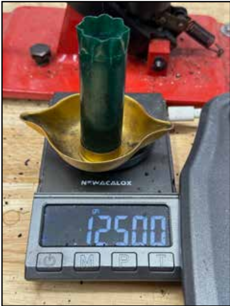
WEIGHING A HULL. REMINGTON HULLS WEIGH AROUND 125 GRAINS.
