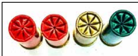
L-R, WIN FACTORY AA; RELOADS — WIN AA, REM STS GOLD, STS GREEN MADE ON DILLON SL900. THE CRIMP IS IMPORTANT.
