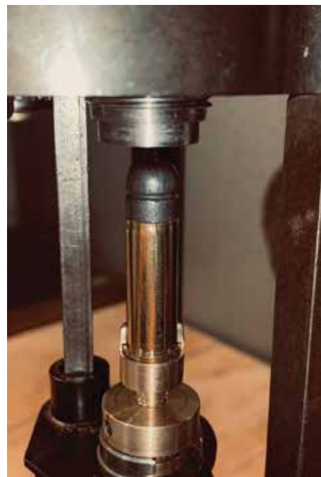
LOADING BEAR CREEK .375 HEELED BULLET WITH OLD WEST BULLET MOLDS' CRIMP DIE.
