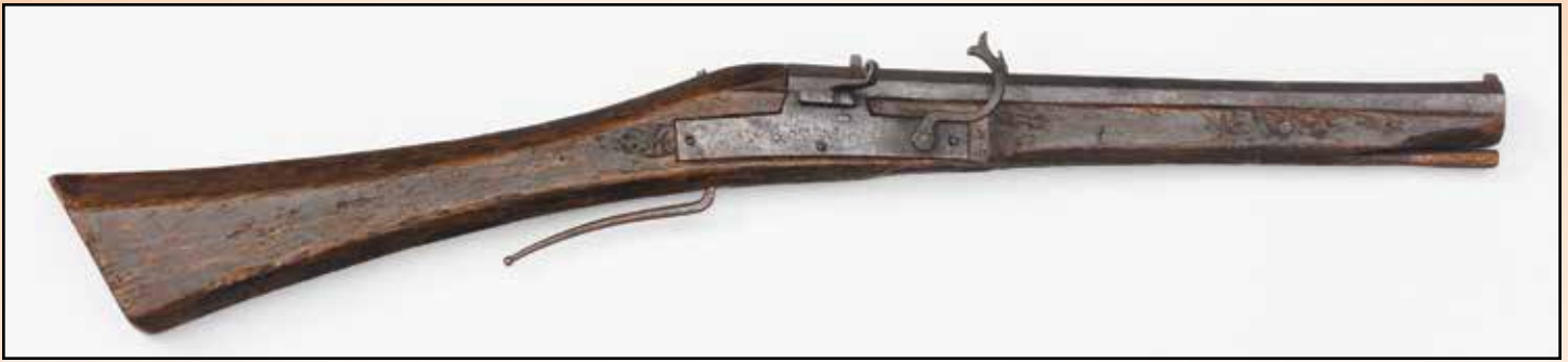
ACCURATE REPLICA OF A GERMAN-MADE MATCHLOCK CARBINE OF THE 1550 PERIOD, WITH A 17-1/4" BARREL OF ABOUT .53 CALIBER. NEARLY IDENTICAL ORIGINALS EXIST THAT HAVE EVEN SHORTER BARRELS. SUCH GUNS WERE WELL-SUITED FOR USE ON HORSEBACK OR ON A WAGON SEAT. —PHOTO COURTESY OF DR. KUNO FISCHER, LUCERNE
